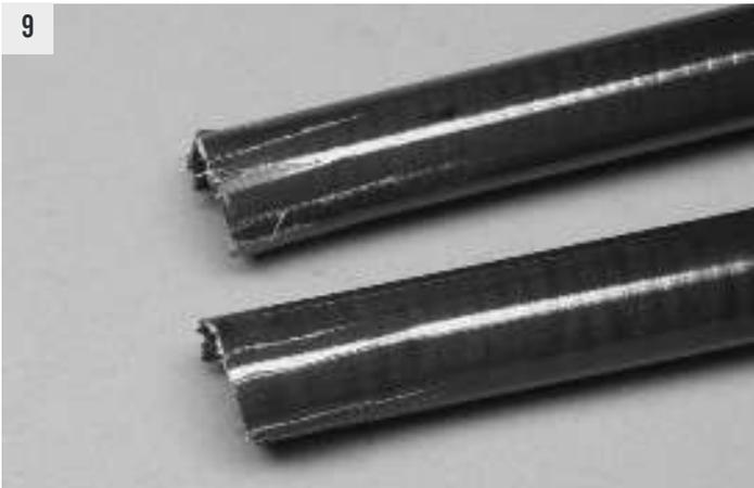
you no longer have a tube and a catastrophic failure is the result. Overload failures are easy to spot. This type of break will always take place in the bottom half of the rod, usually just forward of the handle or the fisherman's furthest point of effort (the rod hand). The break will be slightly irregular with jagged edges and short lengthwise splits and tears (9). Looking at the inside of an overload failure you'll note great distress in the walls of the blank both inside and out (10).
